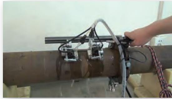
The PA chain crawler CPS-X07 is compatible with PA ultrasonic flaw detector, which is used to perform pipeline corrosion inspection.
